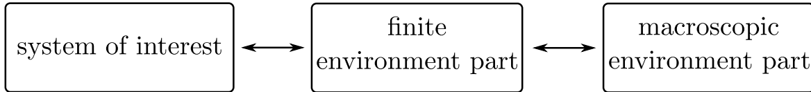
Figure 1.1: Schematic of the nested environment structure harnessed for reservoir engineering throughout this thesis. The system of interest is coupled to a finite environment part, which in turn is coupled to a macroscopic environment part. The environment can be controlled via the finite part, whose dynamics can be tuned.
